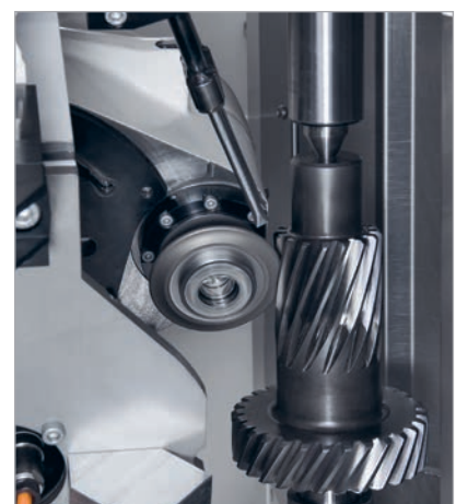
Profile grinding with profile grinding head
