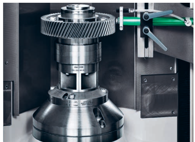
Loading and meshing into grinding position away from the grinding area
