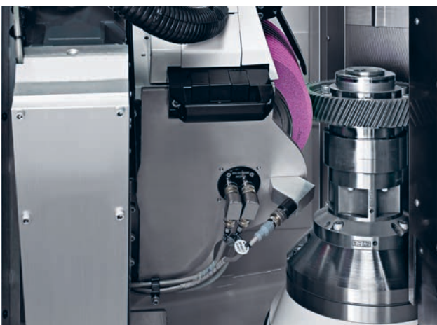
Gear in grinding position
