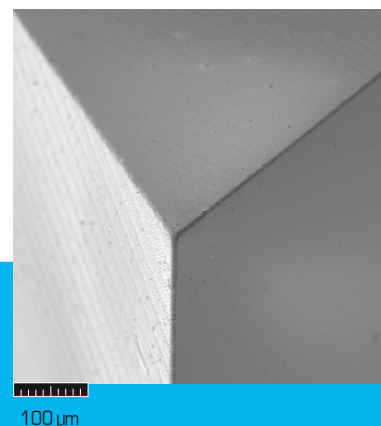
DLC3 coated endmill under scanning electron microscope:
